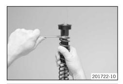
Clamp the open end wrench in the vise. Release screw cap ● but do not remove it yet.
