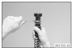
Pull the spring down. Mount the open end wrench on the hexagonal part.
