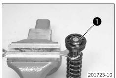
Clamp the open end wrench in the vise. Tighten screw cap ①.
