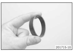
Grind the edges of the sliding bushings with sandpaper grit 600, clean the bushings and lubricate them.
